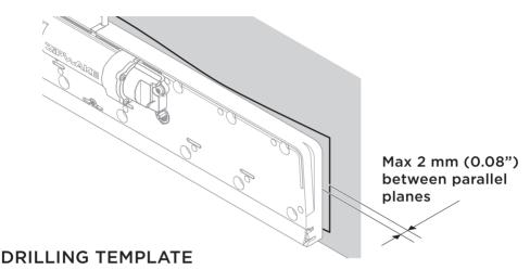
Start mounting the Interceptors as far outward as possible, although well inside the transom. Continue inwards when installing multiple Interceptors.
