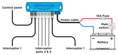
NOTE! The system allows an unpaired Interceptor mounted on the center of the transom. A centerline mounted Interceptor should always be connected to port side 3 to work properly.
